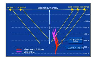
The Caber North deposit (1.3 Mt @ 4.0 % Zn, 1.7% Cu) is buried at > 300 metres depth, under conductive overburden.
