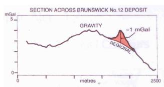
Mafic volcanic rocks produce a large, regional gravimetric Bouguer anomaly. A contrast of density caused by a massive sulphide lens produces a local peak, showing the location of the deposit.
