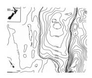
The broad magnetic low with fairly sharp boundaries lies over a recently active geothermal system. The geothermal activity has destroyed the magnetite in the country rock and is responsible for the reduced magnetic intensity in this zone.
