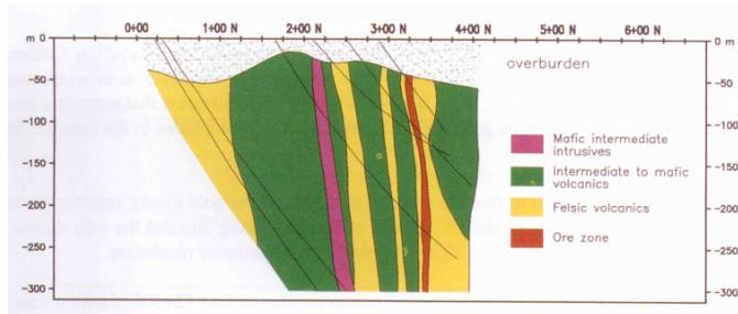
Estrades is a narrow Cu-Zn VMS deposit covered by a layer of conductive overburden, located in the Abitibi Greenstone belt.
