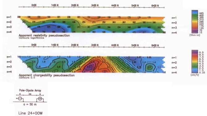
The deposit is clearly detected with IP, but is the resistivity data useful?
