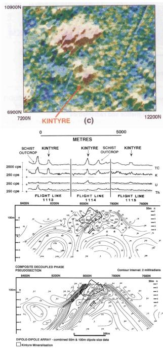
An airborne magnetic/radiometric survey detected elevated counts for K, U and Th at the Kintyre location.
